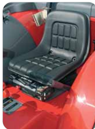
Far left: Spacious and superbly designed. The platform is silent bloc-mounted to minimise noise and vibration.
