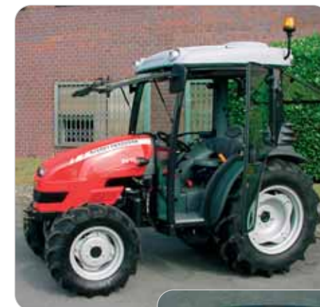
Excellent cab access. Opening front screen and air conditioning give a choice of ventilation options
