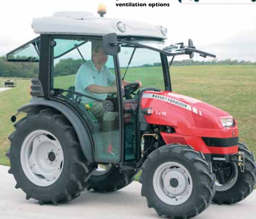
Excellent cab access. Opening front screen and air conditioning give a choice of ventilation options
