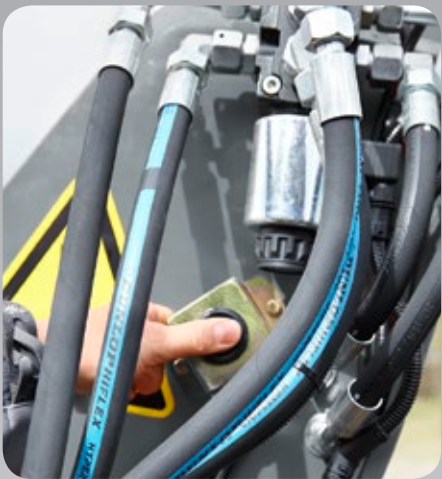
Pressure release of 3rd control circuit (optional). Telehandlers T5522 and T6027 offer a special feature that is helpful for coupling and uncoupling hydraulically operated attachments: the knob for releasing the pressure from the 3rd control circuit is easily accessible from the outside of the telescopic arm. In this way, different attachments can be replaced faster and more efficiently. This works with the ignition switched on or the engine running.
