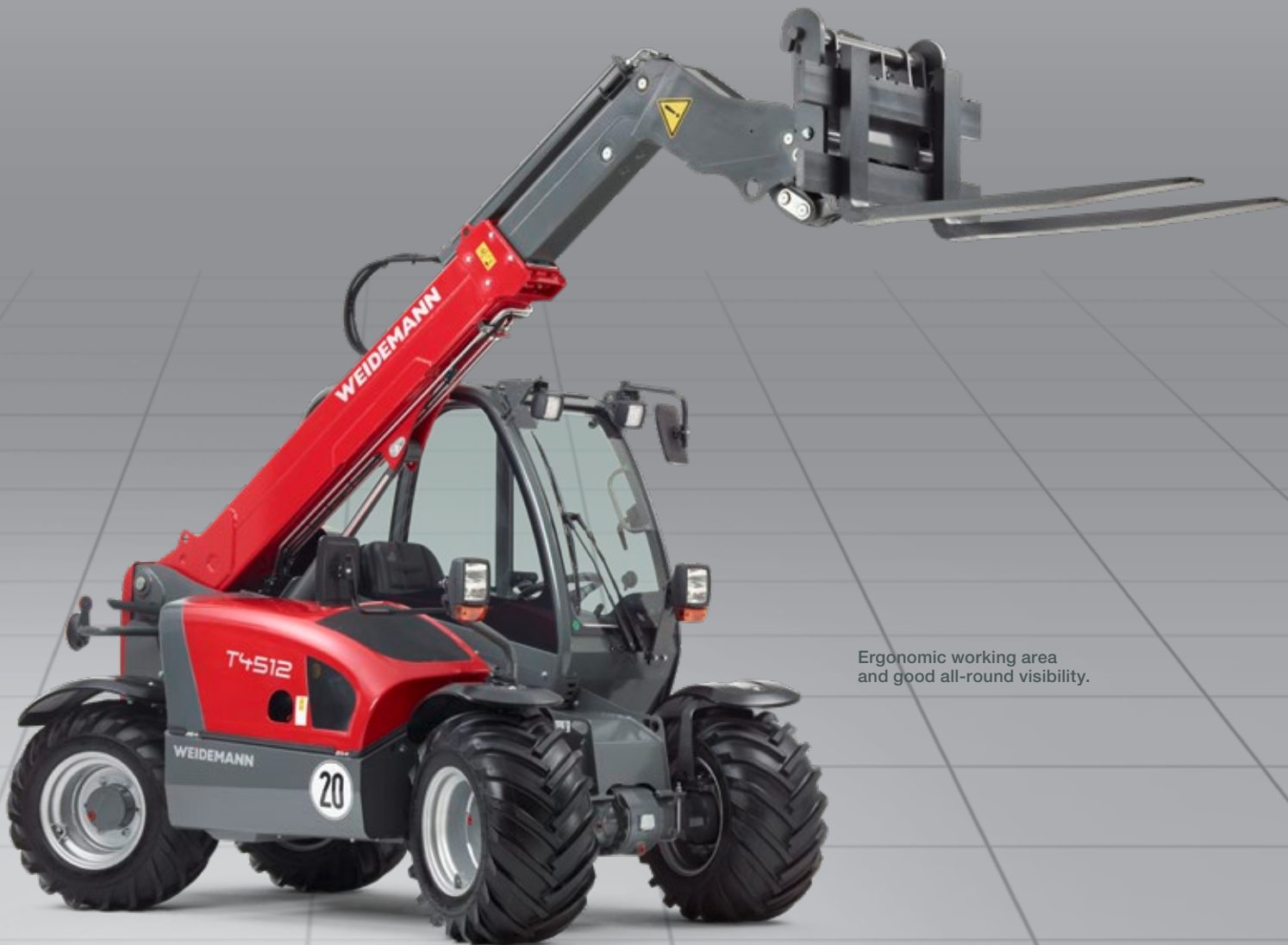
Undivided chassis and all-wheel steering, low center of gravity, and excellent stability.
