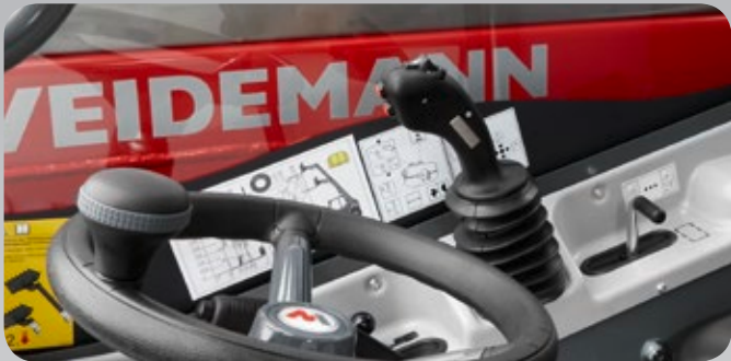
The joystick for the T4512. The joystick helps you to keep the entire machine under control. Sturdy and sensitive control for all lifting and lowering movements and for the tilting out and in of the attachment with just one lever. Optionally, the joystick can be supplemented with additional functions.
