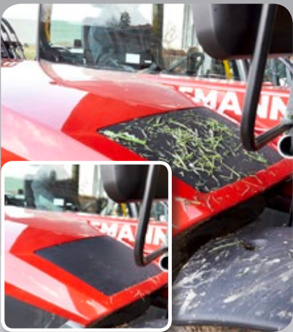
Reversing fan (option for T6027). Contamination of the ventilation grill, e.g. when loading straw, can be counteracted with the reversing fan. The hydraulic motor and pump are designed so that the air flow of the fan can be reversed. The dirt accumulation on the intake surfaces of the engine hood are simply blown away at the push of a button in the cabin.
