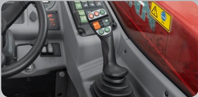
The joystick for T5522 and T6027. The joystick becomes an all-rounder and the machine's ease of use is increased even further. In addition to the functioning of the 3rd proportional control circuit that can be operated on the joystick, the continuous operation of the 3rd control circuit can be activated via a rocker switch – and also in both directions, by moving the thumbwheel. The telescopic function can also be operated proportionally. Both electrical functions can also be operated on the joystick in a detenting or latching manner. Both electric functions are independent so that they can be individually configured by the operator.
