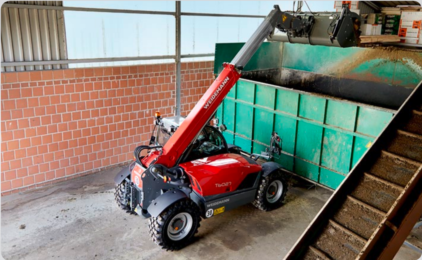
Automatic bucket return (option for T6027). The loading position can be saved by pressing the corresponding button on the joystick. During the next loading process, the attachment can thus be brought back to exactly the same position. The automatic bucket return thus offers extra comfort, precision and speed for the operator for repetitive work, such as stacking or filling bins.
