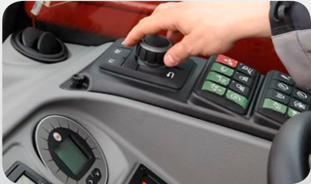
Hydraulic oil volume adjustment (T6027). If necessary, the "jog dial" control element can be used to manually set the flow rate of the hydraulic oil. This is advantageous if the machine is operating a hydraulic attachment that does not require the full hydraulic performance of the machine. The operator can therefore work precisely and in a resource-saving manner with the machine and attachment.
