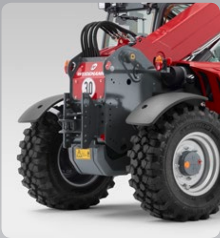
Suitable for trailer operation. Various optional trailer couplings are available: from a simple shunting coupler to a semi-automatic to an auto-hitch trailer coupling (availability depends on model and country).
