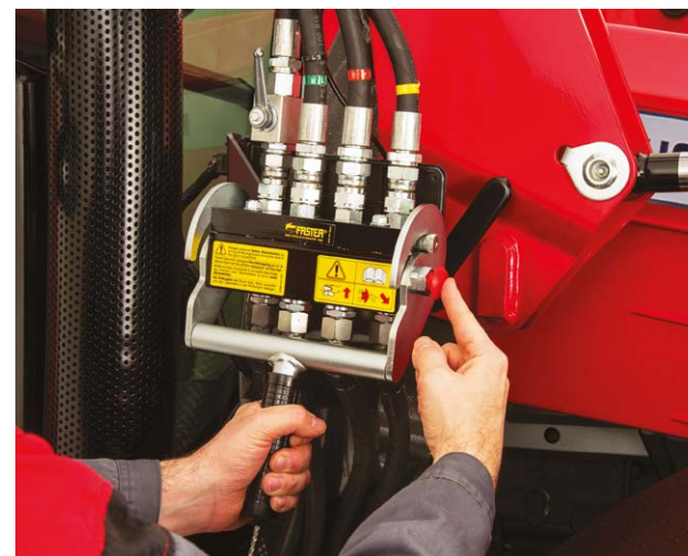
Disconnect the hydraulic and electrical connections
