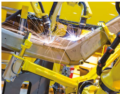
Robotised welding ensures accuracy and strength
